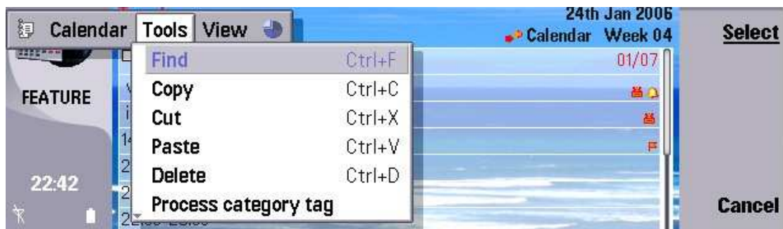
Figure 4: The 'Tools' menu options. The down pointing arrow to the bottom left of the menu indicates further options below – move the cursor down to see them.
