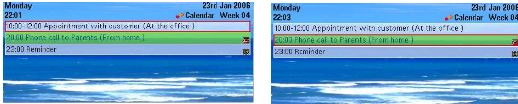
Figure 2: The cursor (in Red) is positioned on the first entry (Left). Moving the cursor down, positions it on the second entry (Right). Pressing enter will enable you to edit the selected entry. The colour of the cursor is customisable in 'Menu/Settings/Colour'
